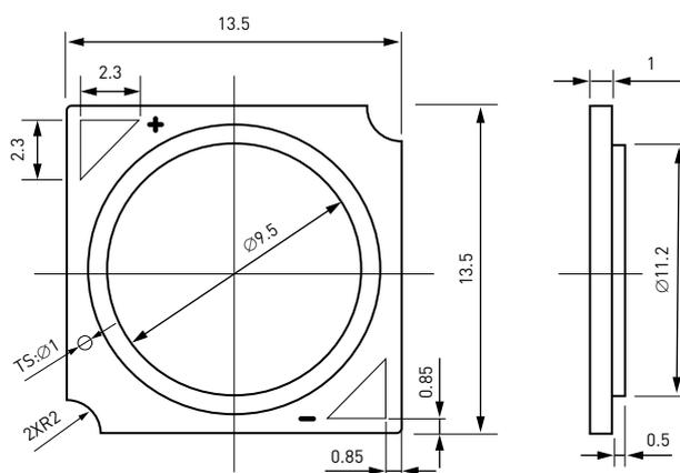
Notes: All dimensions are in millimeters (mm), tolerances are  $\pm 0.3$  mm.
